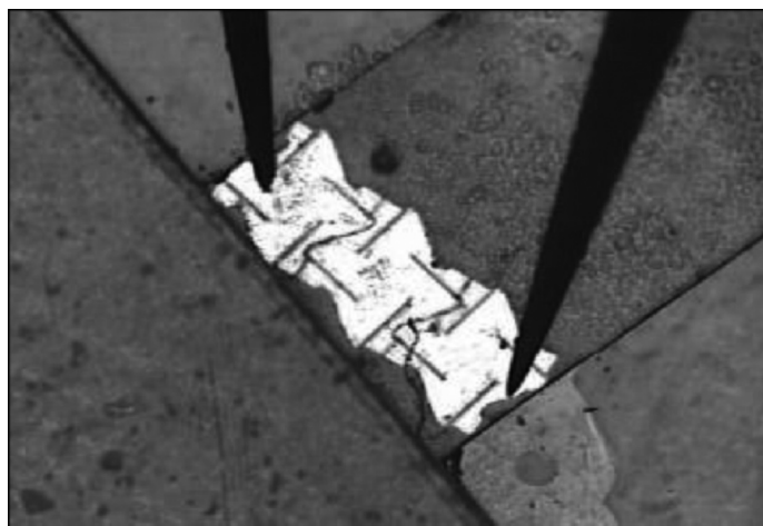
Figure 4: Optical microscope image of resistance measurement across three assembled microtiles.
