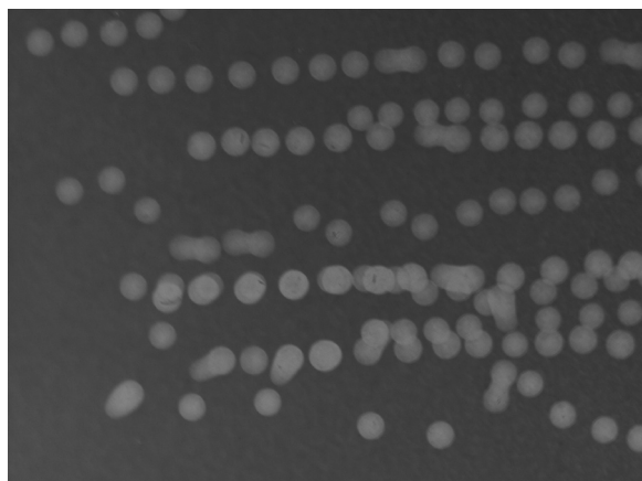
Figure 1: Optical microscope image, PEDOT:PSS on paper at 50 \mu\text{m} drop spacing.
