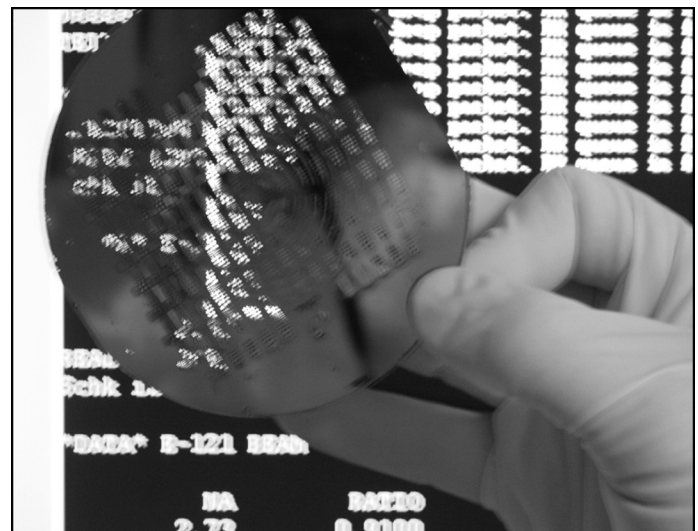
Figure 4, bottom: The computer lights passing through the etched vias in the silicon wafer.
