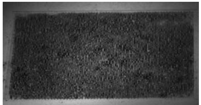
Figure 2, top: 75 \mu\text{m} shallow reservoir device, syringe pumped (photographed using a macro lens).
