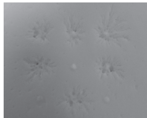
Figure 2: Dendritic structures created in plaster.
