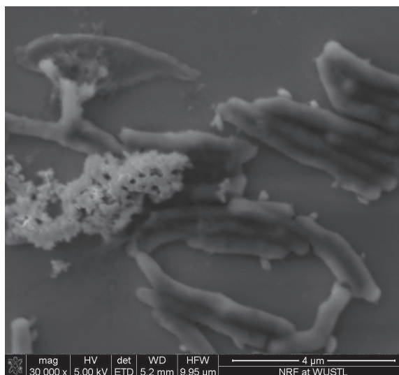
Figure 4: SEM image of M. smegmatis with Cu (3.0%) TiO 2 after UV exposure.
