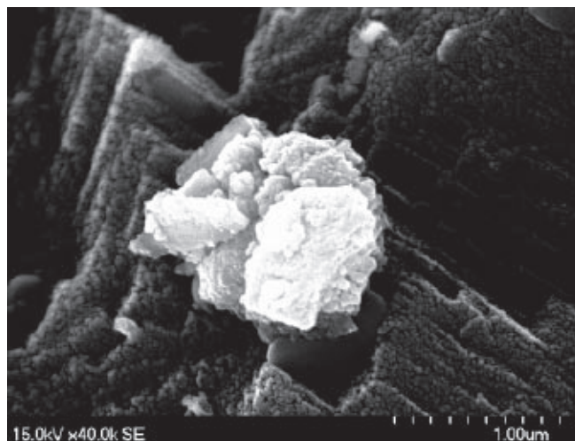
Figure 4: Cluster of magnetite particles on reacted ankerite. Secondary electron image (FE-SEM).
