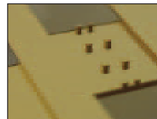
Silicon posts for transitioning a coplanar waveguide ground plane between two wafers (Posts are approximately 1 \mu m square in area.)
