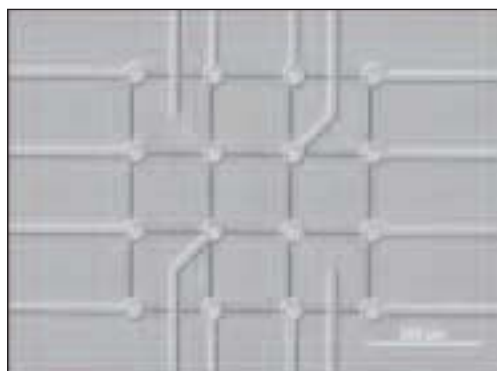
Fabricated multi-electrode array for guided neural growth
