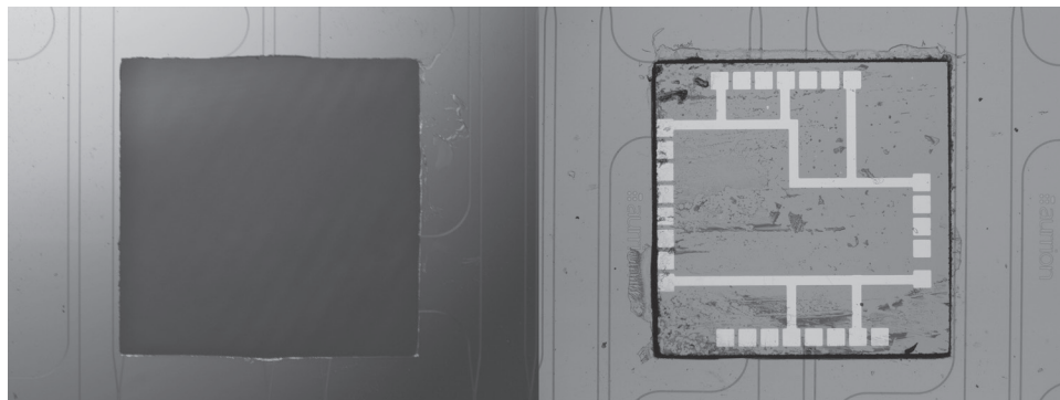
Figure 2: Vacant through-substrate cavity (left) and integrated RLC circuit die (right).
