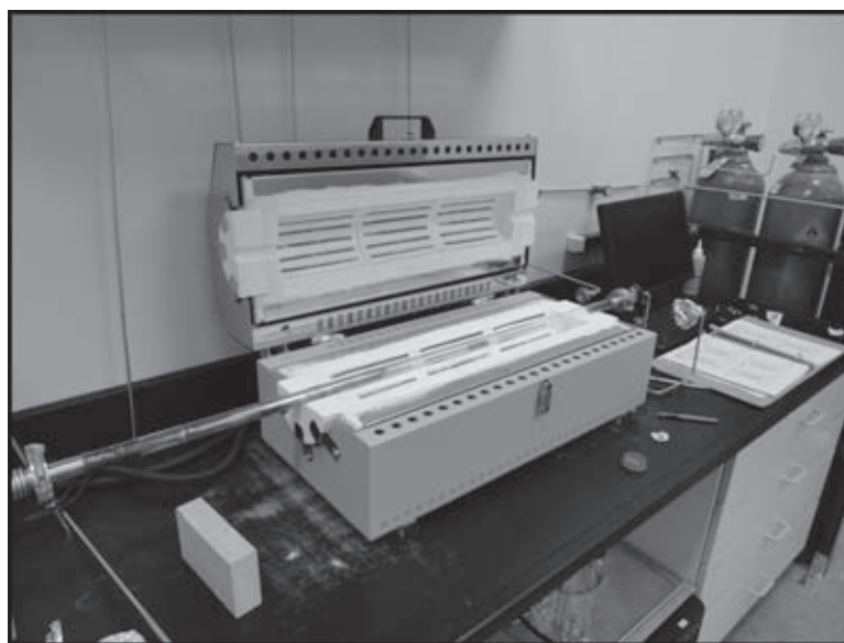
Figure 2, right: Our tube furnace setup where the growth took place, the crucible with \text{Bi}_2\text{Se}_3 at the center of the glass tube.
