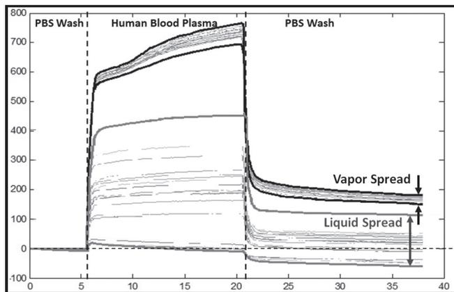
Figure 2: Microring resonator sensorgrams for vapor deposited (black) and liquid deposited (gray) chips. The liquid deposited chip is less uniform (as is apparent by examining the spread in each chip). The standard deviations are  $13 \text{ ng/cm}^2$  and  $123 \text{ ng/cm}^2$  respectively.
