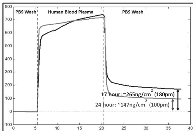
Figure 4: Microring resonator sensorgrams for 17-hour (black) and 24-hour (gray) ATRP reacted chips. These data showed fouling levels of  $265$  and  $147 \text{ ng/cm}^2$  respectively.
