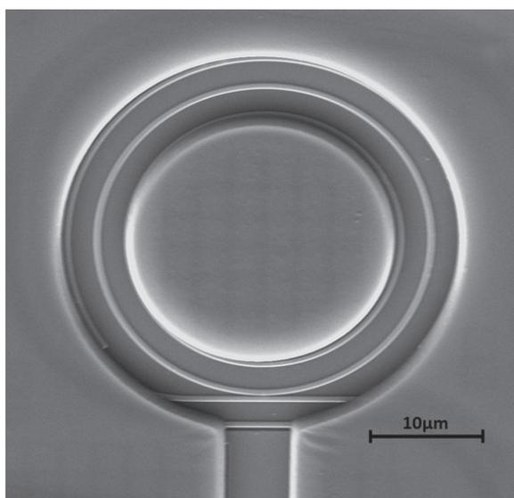
*Figure 1: An SEM image of a microring resonator. Light is directed down a waveguide that runs adjacent to each microring (bottom). Resonance wavelengths are coupled into the microring, causing a decrease in output power.*
