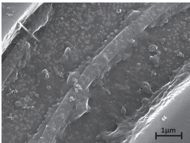
Figure 3: An SEM image of a microring resonator polymerized using liquid initiator deposition. Non-uniform polymer growth was confirmed using this (and other) SEM images.
