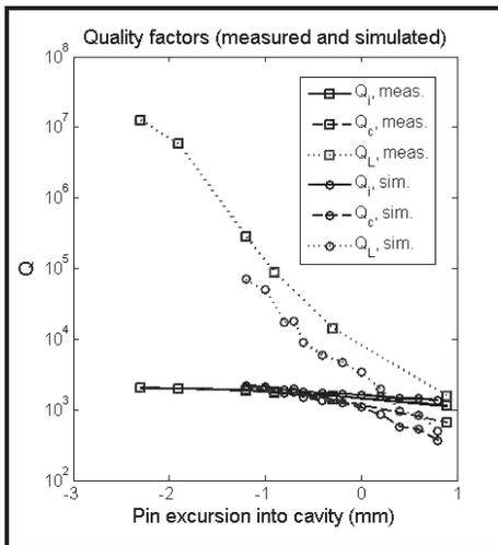
Figure 3: Loaded, intrinsic, and external quality factors as simulated and as measured. In simulation, zero dielectric loss is assumed, and the cavity is defined with bulk conductivity  $3.8 \times 10^7$  S/m.
