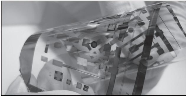
Figure 2: Fabricated devices on flexible substrate.
