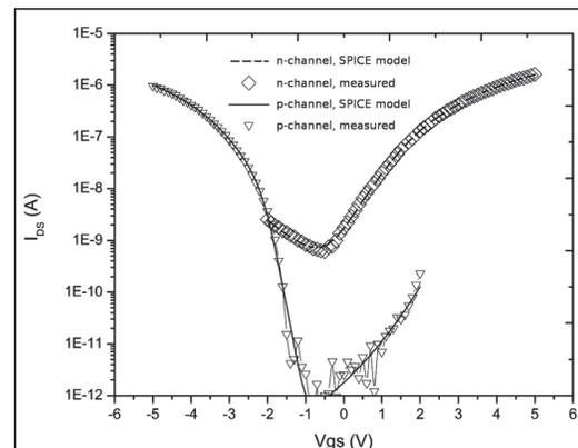
Figure 3, above:  $V_{gs}$ - $I_{ds}$  curves for fabricated devices and for constructed device models.
