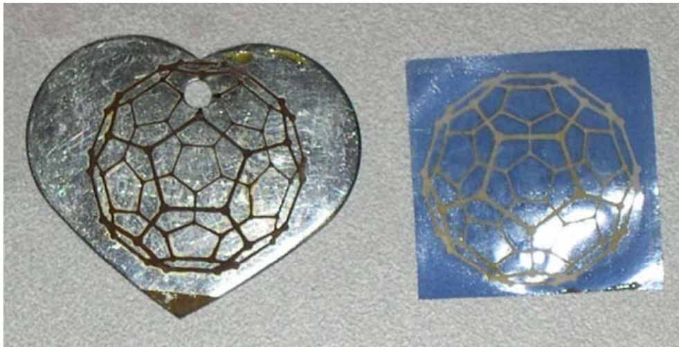
(9) Etched dog tag with oxide pattern and photoresist film.
