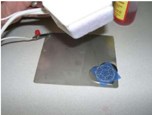
(7) Put electrolyte on photoresist and felt pad; put etcher over dog tag for 10 seconds.
