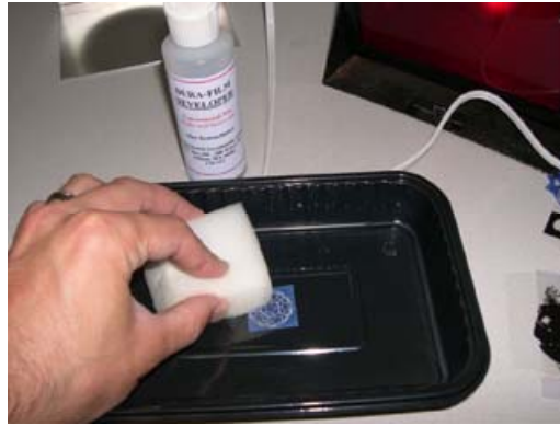
(4) Peel off front and back protective films, then rub blue photoresist with developer for 2 minutes.
