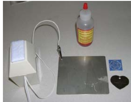
(6) Etch-o-Matic grounding plate, electrolyte, and dog tag to be etched.
