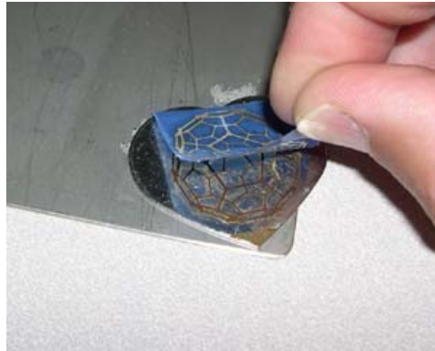
(8) Remove photoresist, rinse and dry.
