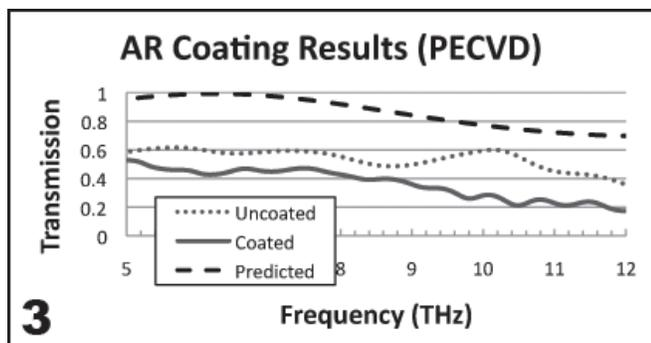
As in the case with e-beam deposition, the  $\text{SiO}_2$  film did not adhere well to the InP sample and flaked off easily. A substantial amount ( $\sim 500$  nm) of bowing was also observed in the coated HR-Si wafers. FTIR spectrometry was used to compare the transmission spectra of the Si wafer before and after deposition. The results are compared to the simulated transmission in Figure 3.
