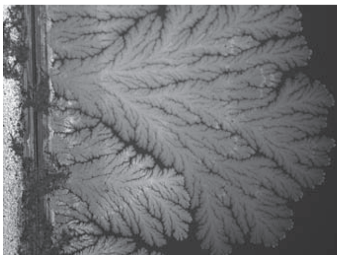
Figure 1: A sample cathode. Dendrites are growing to the left as more silver ions reach the cathode. There are multiple layers of dendrites visible.
