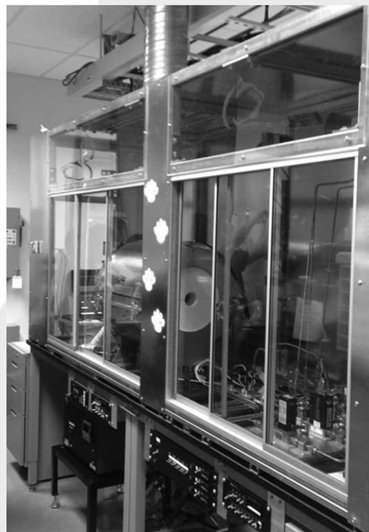
Figure 3, left: Finished MOCVD gas panel and switch box. Figure 4, right: Fully ventilated protective enclosure.
