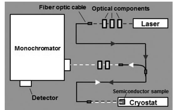
Figure 1: Characterization apparatus diagram. Laser light shown in gray, photoluminescence in white.
