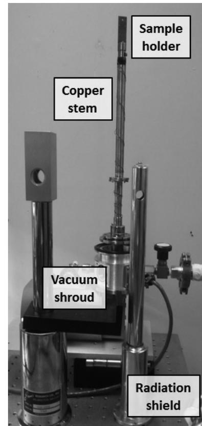
Figure 2: The former cryostat, disassembled. Labeled components were modified.
