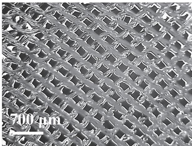
Figure 3: Polyimide and SiO<sub>2</sub> conformation to substrate.
