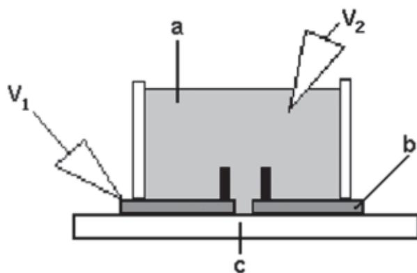
Figure 3: Leakage current testing. (a) Saline solution. (b) Pt electrodes with carbon growths. (c) Silicon substrate.
