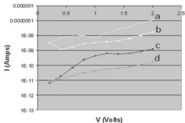
Figure 4: Leakage current data. (a) Uncoated array. (b) 1000/2000Å coating. (c) 1300/5400/1300Å coating. (d) No electrodes (noise).
