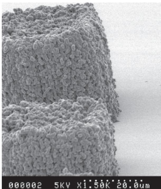
Figure 2: Nanotube pillars coated with 1000Å oxide, 2000Å nitride.
