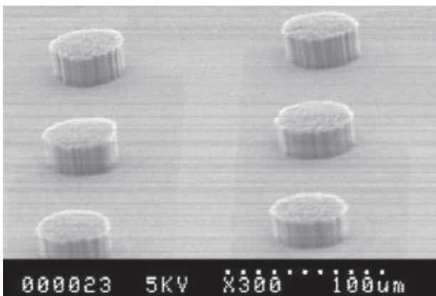
Figure 1: An array of uncoated nanotube pillars.
