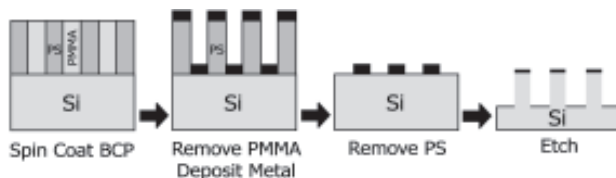
Figure 2: Schematic cross-sectional view of the Block Copolymer Lithography process.
