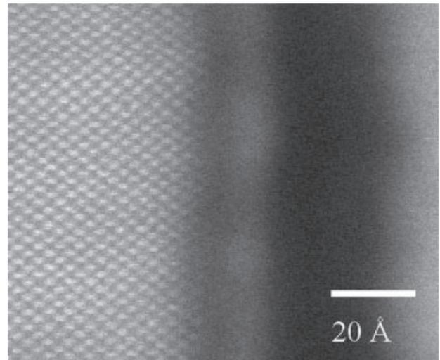
Figure 3: TEM of silicide (center) at Si-Co interface.
