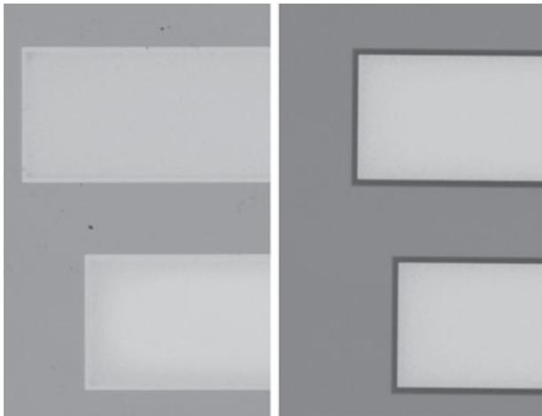
Figure 2: Left: before anneal. Right: after anneal.
