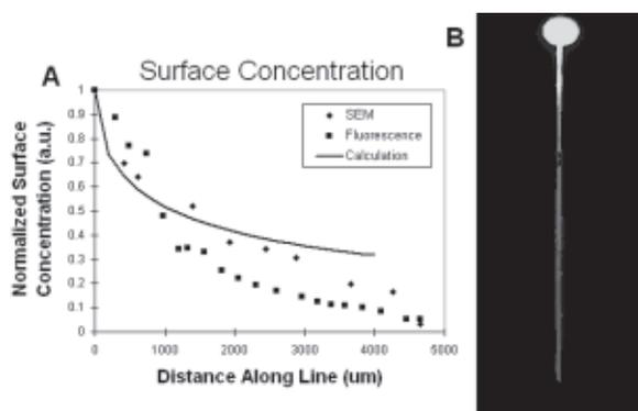
Figure 3: (A) Comparison of SEM and Fluorescent samples with calculation; (B) Fluorescent image of sprayed line.
