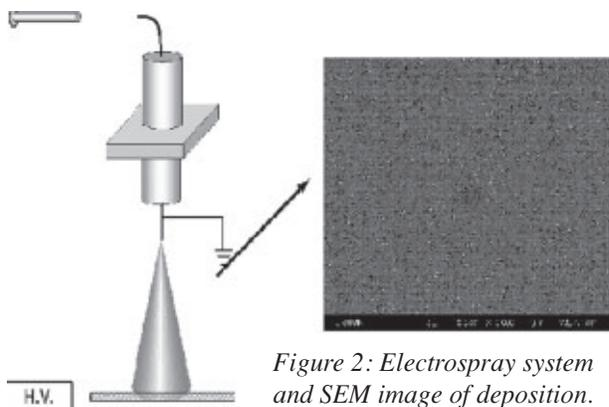
Figure 2: Electrospray system and SEM image of deposition.
