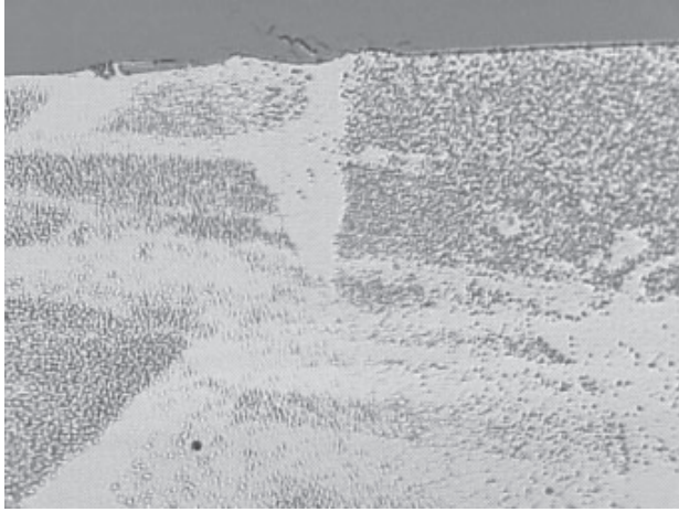
Figure 1: Residue left after incomplete development of resist.
