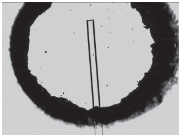
Figure 4: Optical microscope picture of inlet hole over etched silicon channel.
