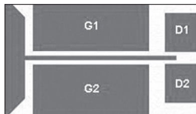
Figure 1: Generalized design for a lateral cantilever beam switch, with a source electrode and two gates (G) and drains (D).
