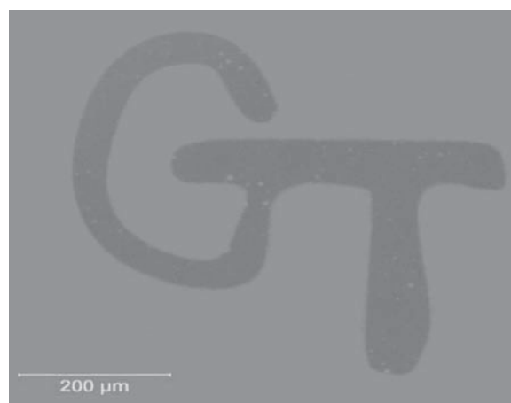
Figure 4: Bioconjugated and photobleached SiO 2 substrate.
