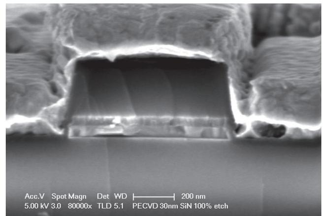
Figure 2: SEM of test structure. The sidewalls appear fairly thin, ~ 30 nm, and conformal to the gate metals.
