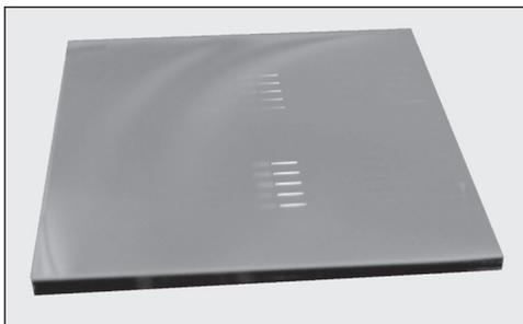
Figure 1: A chip used to test the parameters of the fabrication process.
