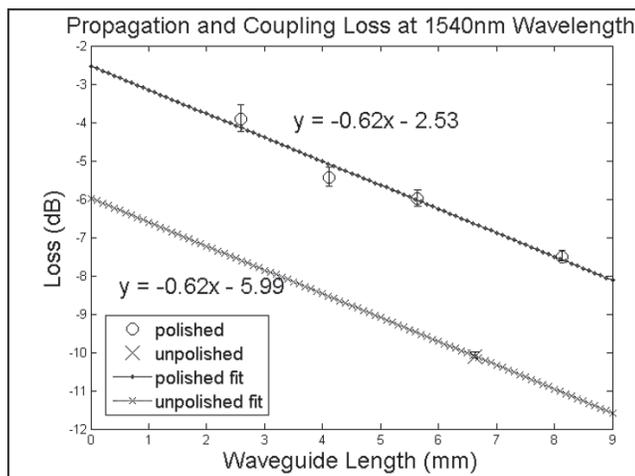
The results, seen in Figure 4, show a propagation loss of 0.62 dB/mm and total coupling losses of 2.53 dB and 5.99 dB, or 1.26 dB and 3.0 dB per each of the two coupling sides, for the polished and unpolished samples respectively. We then successfully pigtailed our device using the plastic holder with a coupling loss faring two times worse than that of an unpigtailed device.
