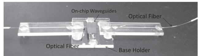
Figure 2: Fiber pigtailed device.
