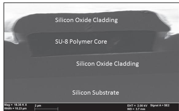
Figure 1: Polished waveguide facet.
