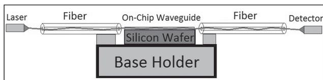
Figure 3, above: Measurement setup.
