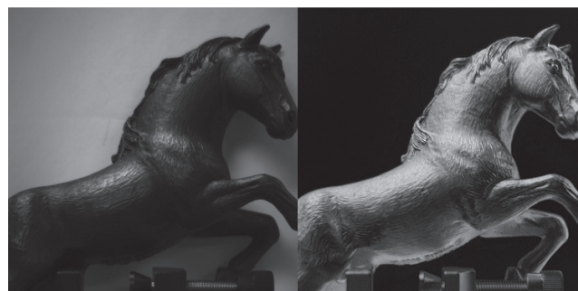
Figure 2: Intensity image of a horse (left) and a polarization image of a horse (right).
