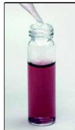
During part I of this lab you will be creating gold nanoparticles (GNP's) approximately 15 nm in size (that's small!). The particles will be covered in a citrate layer that will prevent the gold particles from 'bumping' into each other, sticking and therefore making larger and larger particles. The nanoparticle surfaces can be modified to attach to just about any molecule or antigen. These GNP's will be used to detect simulated meningitis bacteria which will "infect" some of your classmates.
