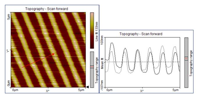
2a. AFM image Sample : Sony DVD-R 4.7 GB; Blank, scan size 5.0 micrometer
