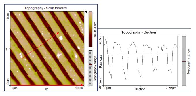
Fig1a. AFM image : Sample : Memorex CD 750 MB; blank; scan size 10 micrometer
