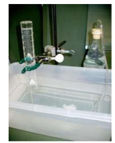
Collecting gas by water displacement
